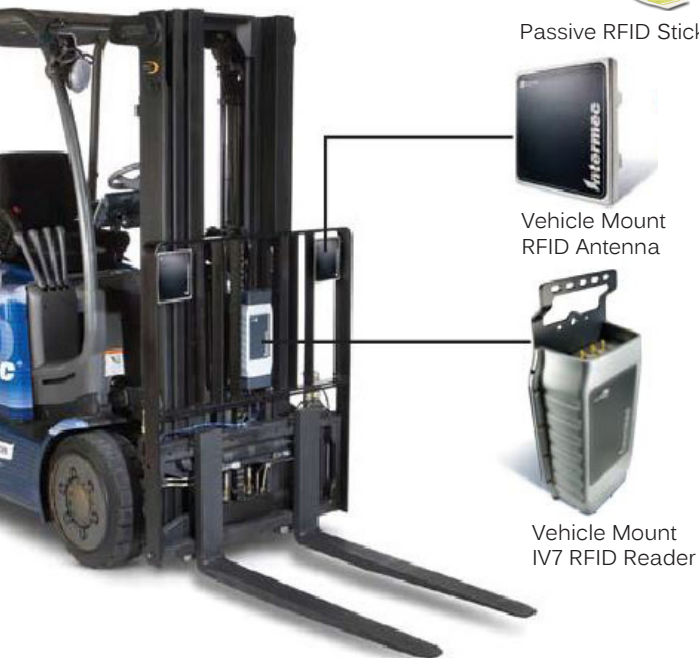
Tracked forklift equipped with vehicle mount RFID reader
