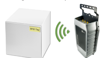
Package identified by RFID Reader
